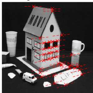
Set 1 Image 2 Using Normalized Eight-Point Algorithm (Rank 2 Enforced) Average Pixel Error= 0.83
